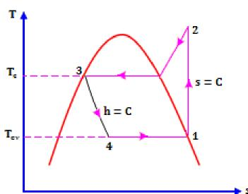
a) Isentropic compression: During the isentropic compression process , the work( $\dot{W}_c$ ) is supplied to the system from the surroundings . There is no change in the entropy in this process .
