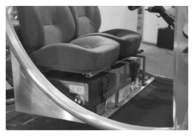
**Figure 3.11** A commercial Zebra battery fitted neatly under the seat of an experimental battery electric vehicle by MES-DEA. The battery stores about 18 kWh of electrical energy
