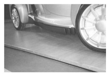
Figure 5.22 Solid metal cooling fins on the side of a GM Hy-wire demonstration fuel cell vehicle
