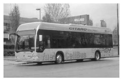
**Figure 1.17** Citaro fuel-cell-powered bus, one of a fleet that entered service in 2003 (Photograph reproduced by kind permission of Ballard Power Systems)
