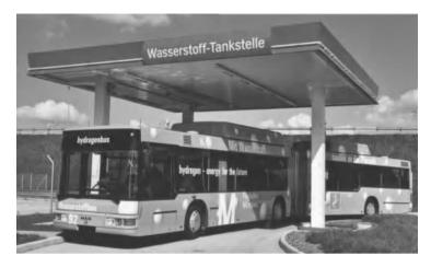
**Figure 6.2** A hydrogen filling station. The bus in the picture is not electric, but uses a hydrogen-fuelled IC engine (Picture kindly supplied by MAN Nutzfahrtzeuge A.G.)
