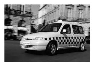
**Figure 14.4** Peugeot 'Partner' battery electric van (Photograph reproduced by kind permission of Peugeot)
