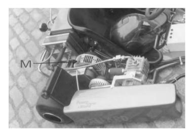
Figure 7.4 Small ( $10 \,\mathrm{kW}$ ) DC 'Lynch'-type DC motor, which is labelled M. This go-kart is fuel cell powered. The unit in front of the motor is the air pump, which is driven by its own motor – a smaller version of the traction motor
