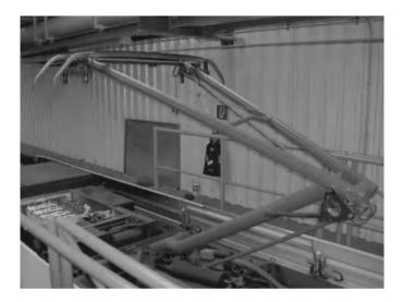
Figure 4.4 Overhead pantograph. (Source: http://en.wikipedia.org/wiki/Pantograph\_(rail).)
