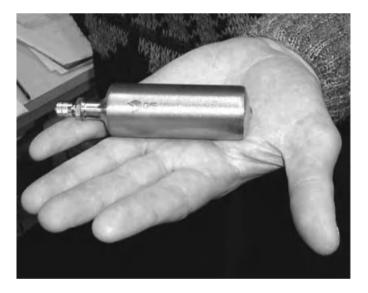
**Figure 6.5** Metal hydride stores can be made quite small, as this example shows
