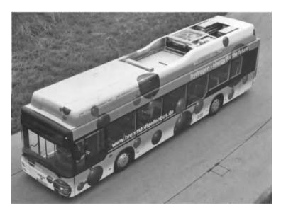
**Figure 5.2** A fuel-cell-powered bus in use in Germany. Vehicles like this, used all day in cities, and refuelling at one place, are particularly suited to being fuel cell powered. (Reproduced by kind permission of MAN Nutzfahrzeuge AG.)
