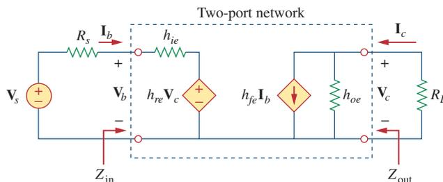
**Figure 19.57** Transistor amplifier with source and load resistance.
