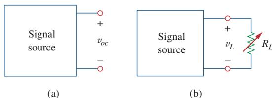
**Figure 4.61**(a) Measuring  $v_{oc}$ , (b) measuring  $v_L$ .
