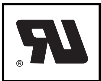
Figure 1-8 The recognized components mark.
