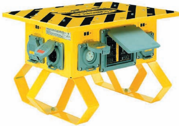
Figure 6-20 A temporary power box used on construction sites. This particular type is connected with a 50-ampere, 120/240-volt power cord. It has six 20-ampere, GFCI-protected, 125-volt receptacles plus additional 30-ampere and 50-ampere Twist-Lock® receptacles. Courtesy of Hubbell Incorporated, Wiring Device Division.
