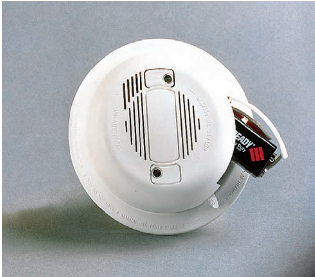
Figure 26-3 An ac-dc smoke alarm that operates on 120 volts ac as the primary source of power and a 9-volt battery as the secondary source of power. In the event of a power outage, the alarm continues to operate on the battery. Courtesy of BRK Electronics.
