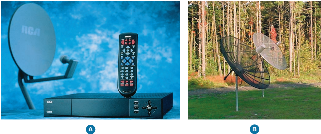
Figure 25-6 (A) A digital satellite system 18-in. (450 mm) antenna, a receiver, and a remote control. (B) A large satellite antenna securely mounted to a post that is anchored in the ground. These large antennas are rarely used today.
