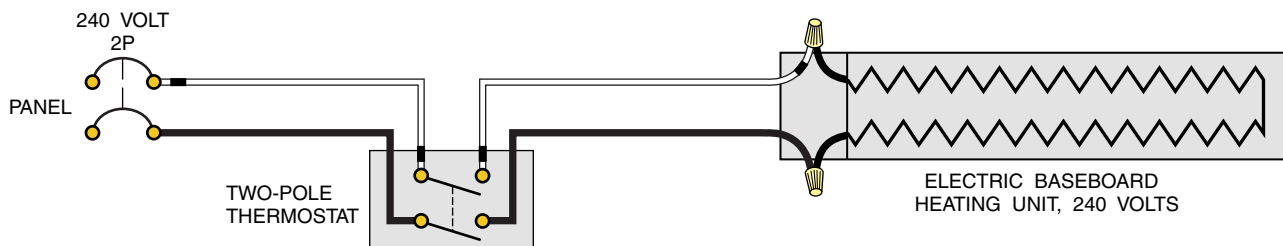
Figure 23-5 Wiring for a single electric baseboard heating unit. The thermostat is a line-voltage thermostat. See Figure 23-3 caption for color-coding requirements.
