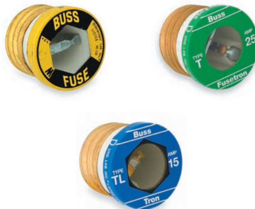
Figure 28-7 Three types of plug fuses: single-element, nontime-delay (W); dual-element, time-delay (T); loaded link, time-delay (TL). Courtesy of Cooper Bussmann, Inc.
