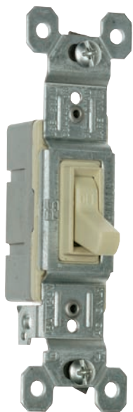
Figure 5-32 Single-pole toggle switch. Note that this switch has a terminal for the connection of an equipment ground conductor. Thus, when a metal faceplate is installed, it will be grounded. See 404.9(A) and (B). Courtesy of Pass & Seymour.
