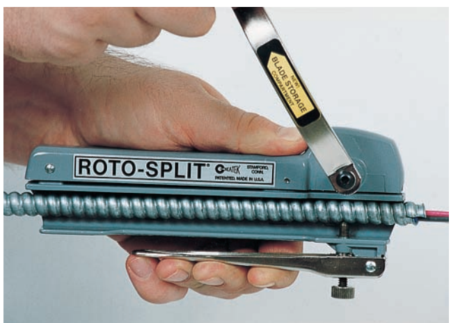
Figure 4-24 This is an example of a tool that precisely cuts the outer armor of armored cable, making it easy to remove the armor with a few turns of the handle. Courtesy of Seatek Co., Inc.
