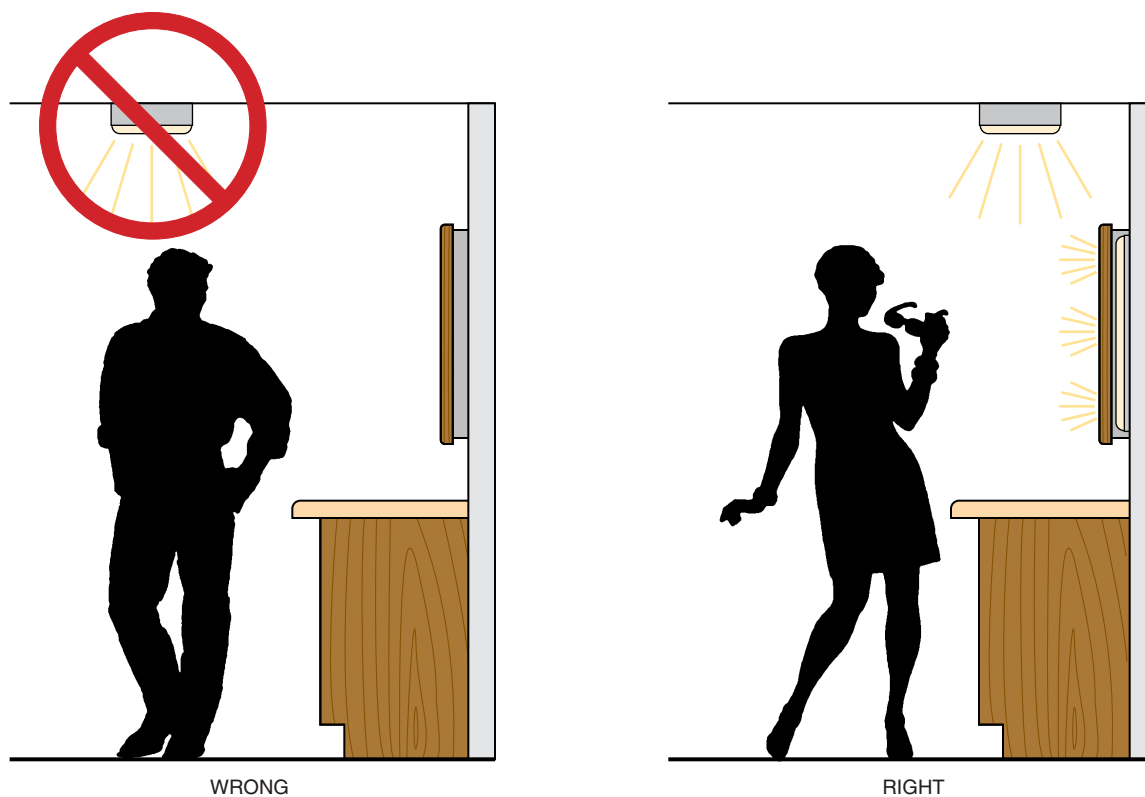
Figure 10-4 Positioning of bathroom luminaires. Note the wrong way and the right way to achieve proper lighting.
