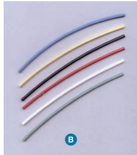
Figure 5-2 (A) Shows a white conductor reidentified with black plastic electrical tape. (B) Shows an assortment of easy-to-use, 6-in. long heat shrink tubing that is slid over the conductor to be reidentified, then shrunk tightly over the conductor by applying heat as specified in the instructions.
