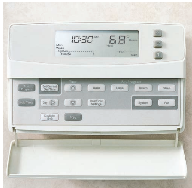
Figure 24-7 A digital electronic programmable thermostat that provides proper cycling of the heating system, resulting in comfort as well as energy savings. This type of thermostat, depending on the model, can be programmed to control temperature, time of operation, humidity, ventilation, filtration, circulation of air, and zone control. Installation and operational instructions are furnished with the thermostat. Courtesy of Honeywell, Inc.
