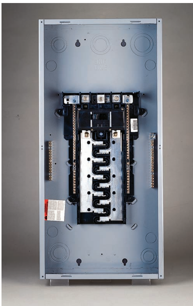
Figure 27-10 A typical 120/240-volt, single-phase, 3-wire load center. This load center has a main circuit breaker. Note the neutral terminal strips on which to terminate the white branch-circuit grounded conductors, and the equipment grounding terminal strips on which to terminate the equipment grounding conductors of nonmetallic-sheathed cable. See 230.66. Courtesy of Schneider Electric.
