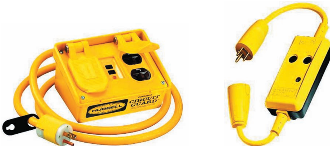
Figure 6-21 Plug- and cord-connected “portable” GFCI devices are easy to carry around. They can be used anywhere when working with electrical tools and extension cords. These devices operate independently and are not dependent upon whether or not the branch circuit is GFCI protected. These portable GFCI in-line cords are relatively inexpensive and should always be used when using portable electric tools. Courtesy of Hubbell Incorporated, Wiring Device Division.
