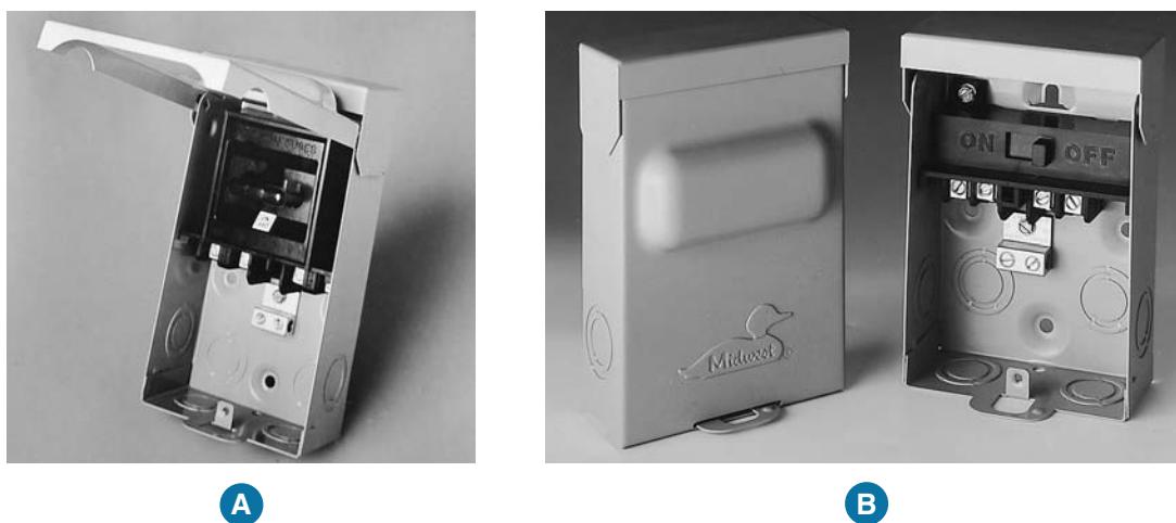
Figure 23-18 (A) is a pull-out fusible disconnect. Fuses are inserted into fuse clips on the pull-out device. Insert the pull-out device for “ON,” and remove the pull-out device for “OFF.” (B) is a nonfusible disconnect, available in 30- and 60-ampere ratings at 240 volts. Both have padlock provisions to prevent unauthorized tampering. Air-conditioner disconnects are available that have a GFCI receptacle as part of the disconnect enclosure. The GFCI receptacle must be wired to a separate 20-ampere, 120-volt branch circuit. Courtesy of Midwest Electric Products.
