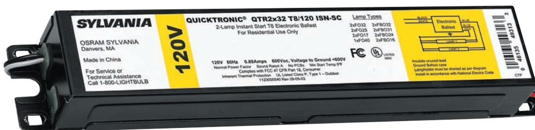
Figure 7-13 An electronic Class P ballast, thermally protected as required in 410.130(E). Electronic ballasts provide improved performance in fluorescent lighting installations. Electronic ballast lighting systems are 25–40% more energy efficient than conventional magnetic (core & coil) ballast fluorescent systems. Courtesy of OSRAM Sylvania.
