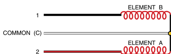
Figure 20-7 Typical surface unit wiring.
