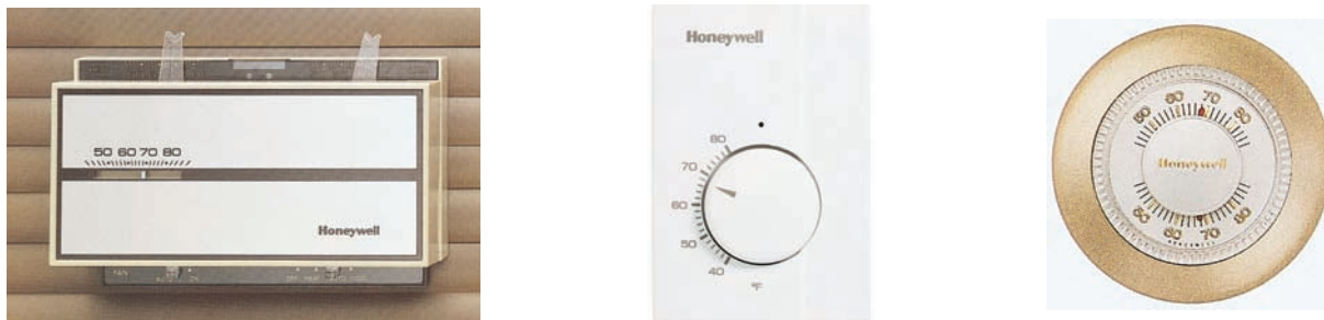
Figure 23-2 Thermostats for electric heating systems. A thermostat or other switching device that is marked with an “OFF” position must open all ungrounded conductors of the circuit when turned to the “OFF” position. Typical mounting height is 52 in. (1.3 m) to center. Courtesy of Honeywell, Inc.
