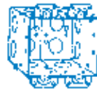
GANG SECTIONAL BOXES TOGETHER TO FORM LARGER BOXES
